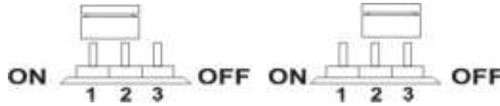
Chart 4-5 Switch for start-up Program Protection Battery
